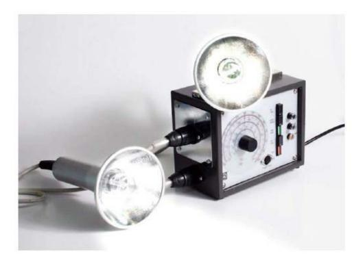
used for rotating and vibrating speed measurement as well as for the observation of fast moving periodic or non-periodic mechanisms at two from each other separately located fields of events at the same time; for instance in printing, paper, labelling and packaging industry etc.
